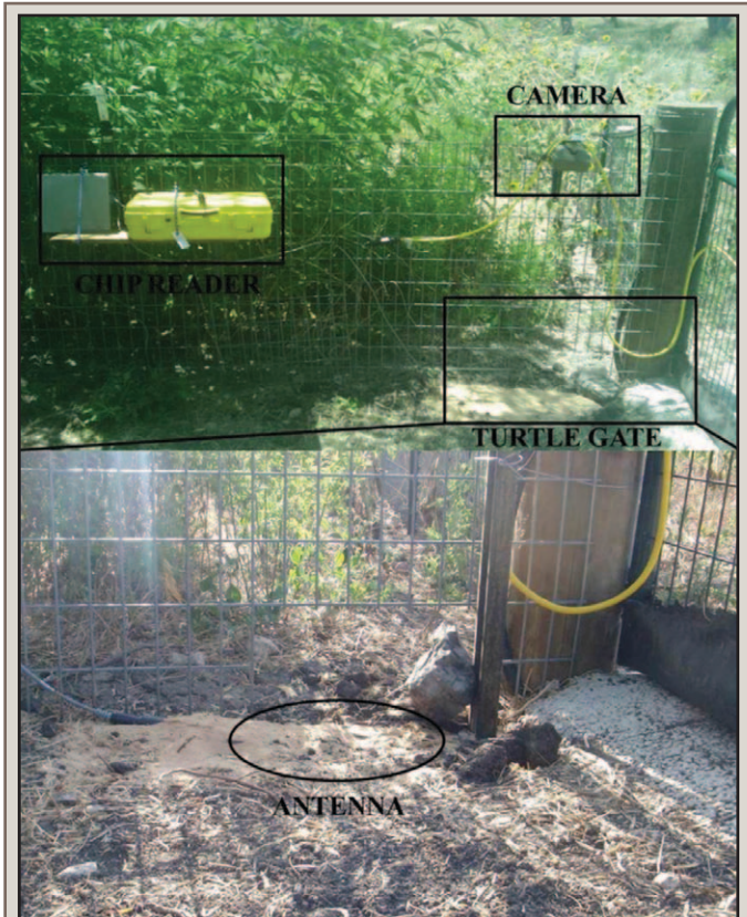
FIG. 2. Stationary reader system placed at the only opening (turtle gate) of otherwise enclosed area (Enclosure Pond 1). While the reader scanned PIT-tagged turtles that pass through the gate, the game camera recorded the images and the direction of the movement.
